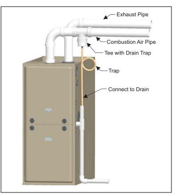
FIGURE 26: Typical. Combustion Pipe Drain Tee.
