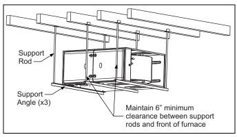
FIGURE 5: Typical Suspended Furnace / Crawl Space Installation
