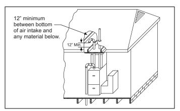
FIGURE 41: Attic and Crawl Space Combustion Air Termination
