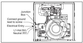
FIGURE 18: Electrical Wiring
