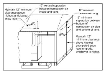
FIGURE 34: Termination Configuration - 2 Pipe
