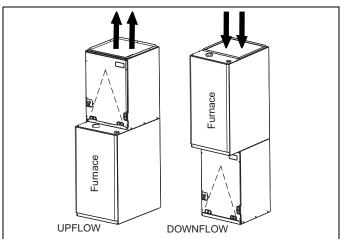
FIGURE 8: Vertical Applications (Typical)
