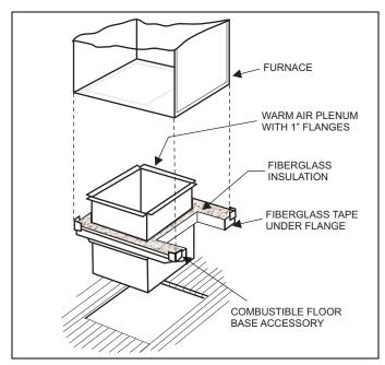
FIGURE 2: Combustible Floor Base Accessory
