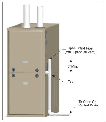
FIGURE 25: Typical. Condensate drain, vertical installation.
