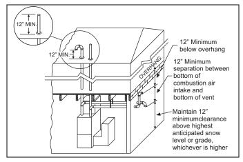
FIGURE 35: Termination Configuration - 2 Pipe Basement
