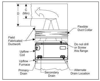
FIGURE 12: PC Series Upflow Coil Installation
