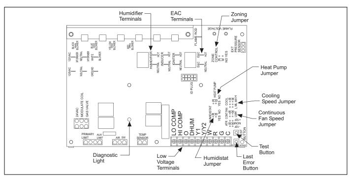
FIGURE 43: Furnace Control Board
