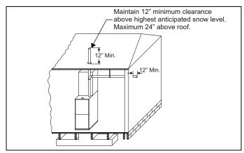
FIGURE 33: Termination Configuration - 1 Pipe
