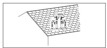
FIGURE 37: Double Vertical Combustion Air Intake and Vent Termination
