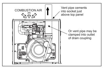
FIGURE 39: Combustion Airflow Path Through The Furnace Casing
