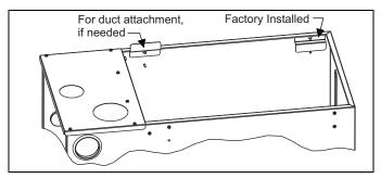
FIGURE 1: Duct Attachment
