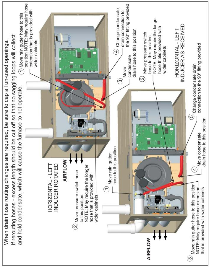
FIGURE 29: Horizontal Left Configuration
