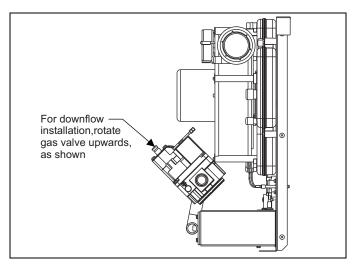
FIGURE 7: Downflow Installation - Gas Valve Rotation
