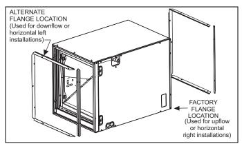
FIGURE 9: Coil Flange
