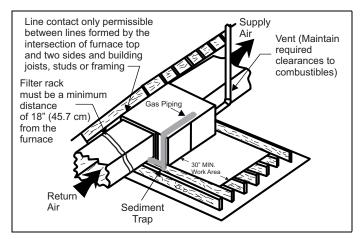
FIGURE 4: Typical Attic Installation
