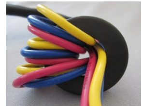
FERRITE WITH UNIT WIRING INSTALLED
