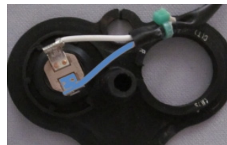
COMPRESSOR OVERLOAD (SAT)
