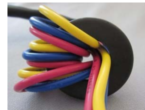
FERRITE WITH UNIT WIRING INSTALLED
