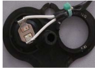
COMPRESSOR OVERLOAD ASSEMBLY (SAT)
