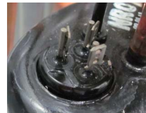
COMPRESSOR TERMINALS (U, V, W)
