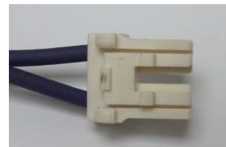
POWER CONNECTOR FOR REVERSING VALVE (TYPICALLY PLUGGED INTO THE OUTDOOR CONTROL 4V JACK)
