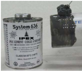
Cement Exterior of Pipe
